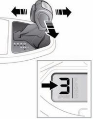
To use CommandShift<sup>™</sup>, first select sport mode, then move the selector lever forward to move up a gear, and back to move down gear.
