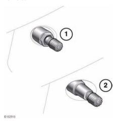
Wheels fitted with a TPM system can be identified by the appearance of the external metal lock nut and valve (1). All Land Rover non-TPM system wheels have a rubber valve fitted (2).
