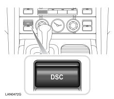
To deactivate DSC, press the DSC switch on the facia (the DSC warning indicator will illuminate continuously). Deactivating DSC has no affect on traction control operation.
