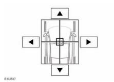
Touch the arrow soft keys to move the sound focal point to the desired area of the vehicle (the focal cross-hairs will appear red when not in the default position).
