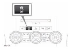
To disable DSC, press and briefly hold the DSC OFF switch on the fascia (the DSC off warning lamp will illuminate continuously).
