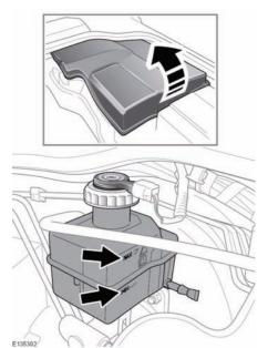
The right hand under-hood cover (as viewed from the front of the vehicle) must be removed to check the brake fluid level, See 161, UNDER HOOD COVERS - REMOVAL.
