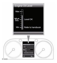
If the oil level is within the required operating range, the message **Engine Oil Level OK** will be displayed. Do not add any additional oil to the engine.
