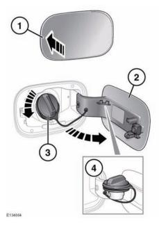
The fuel filler flap is located on the right-hand side of the vehicle, at the rear.
