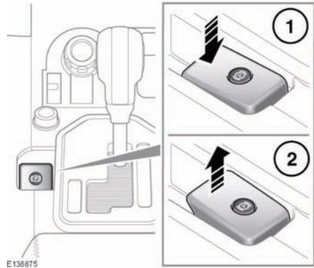
The switch which operates the parking brake is mounted on the center console to the left side of the gear selector.
