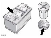
Unscrew the six cell plugs and store carefully. Check that the surface of the battery fluid is level with the plastic level indicator. If necessary, top up with distilled water, but never overfill. Refit the six cell plugs.
