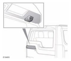
When reverse gear is selected, the touch screen automatically displays a wide angle, color image from the rear of your vehicle.
