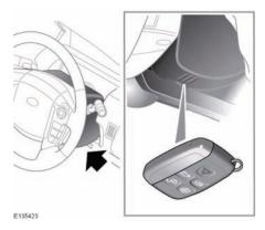
Position the Smart Key against the underside of the steering column cover with the buttons facing downwards.
