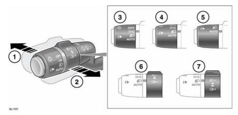
With the headlamps on, push the control away from the steering wheel to select high beam. The instrument pack warning lamp will illuminate.
