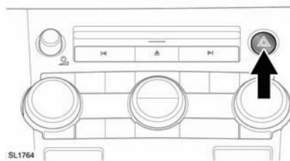
Press to turn the hazard warning lamps on. Press again to turn off. When the hazard warning lamps are operating, the direction indicator warning lamps will flash in time with the hazard warning lamps.
