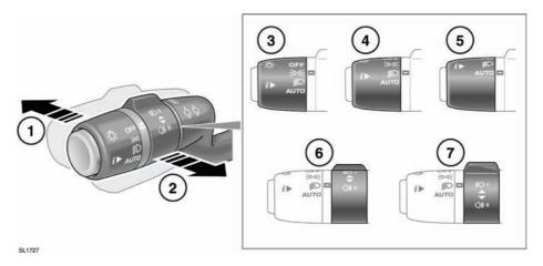
1. With the headlamps on, push the control away from the steering wheel to select high beam. The instrument pack warning lamp will illuminate.
