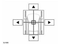
Touch the arrows to move the sound focal point to the desired area of the vehicle.
