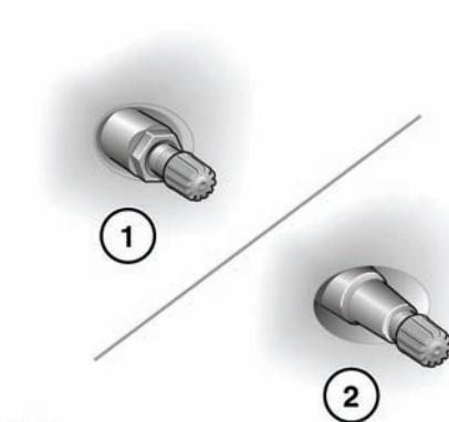
1. TPM system external metal lock nut and valve.
