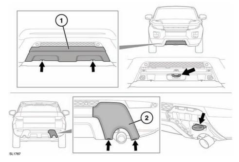
The towing points are located behind panels in the bumpers. Panel design will vary depending on the vehicle specification.
