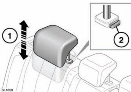
1. To raise, pull the restraint upwards.
