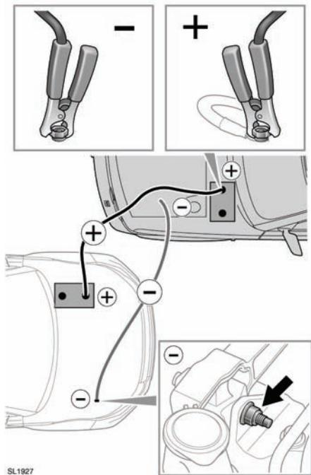
1. Connect the positive (Red) booster cable to the positive (+) terminal on the donor vehicle's battery.
