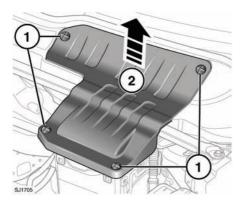
**1.** Turn the four fasteners 90 degrees counter-clockwise to release.
