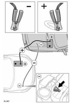
Connect the positive (Red) booster cable to the positive (+) terminal on the donor vehicle's battery.
