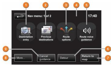
Note: To access navigation press either the NAV hardkey on the surround or touch the Navigation icon on the touch screen.
