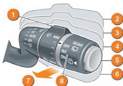
If freezing conditions are likely, the wipers can be set to a higher position so that they can be lifted from the screen. See page 6, **Vehicle information and settings menu**.
