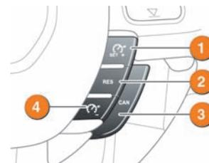
1. Press when the desired speed is reached or to increase speed in 1mph (2 km/h) increments.
