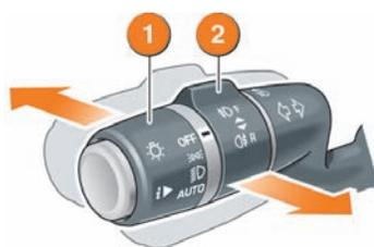
**1. Outer collar.** First position for sidelamps, second position for headlamps, third position for **AUTO**. With **AUTO** selected, all lamps will switch on when exterior light fades to a pre determined level.
