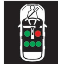
A warning graphic on the instrument panel will illuminate if a seat belt is unbuckled. This will be accompanied by a message in the driver information center.
