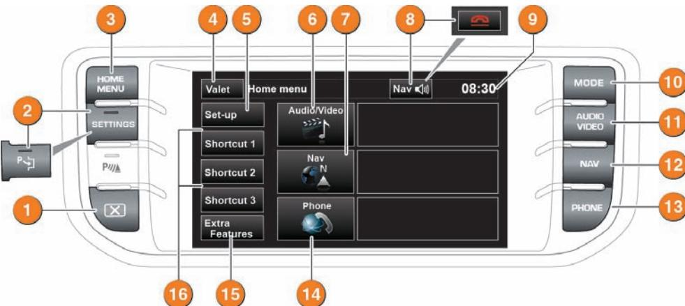
1. Screen on/off. Each time the ignition is turned on and this button is pressed, the **Home menu** will be displayed. If the ignition remains on and the touch screen is turned off and later turned on again, the last used screen or menu will be displayed.
