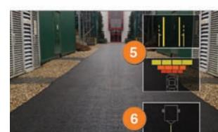
6. Hitch assist. Designed to aid the process of guiding the vehicle to the trailer tow hitch. A single hitch line is displayed as the reversing guideline. As the vehicle closes to within 23.5 inches (0.6m) of the tow hitch, an automated zoom is operated.
