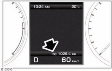
A short press (1 second or less) or a series of short presses of the **i** button will change the trip computer display. The options available are:
