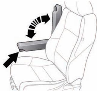
The folding armrest may be stowed by moving to the vertical position. Use the adjuster wheel (arrowed) to set the required height.
