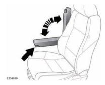
The folding armrest may be stowed by moving to the vertical position. Use the adjuster wheel (arrowed) to set the required height.
