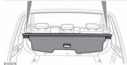
1. With the cover retracted, press the release button on the right-hand end of the cover cassette.
