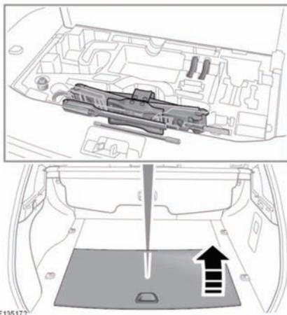
The tool kit is located under a panel set in the loadspace floor.
