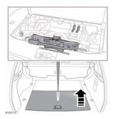
The tool kit is located under a panel set in the loadspace floor.
