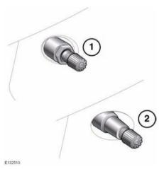
Wheels fitted with a TPMS can be identified by the appearance of the external metal lock nut and valve (1). All Land Rover non-TPMS wheels have a rubber valve fitted (2).
