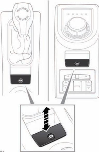
With the ignition turned on, press the brake pedal and press down on the EPB switch. This will release the electronic parking brake.
