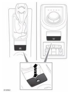
With the ignition turned on, press the brake pedal and press down on the EPB switch. This will release the electronic parking brake.
