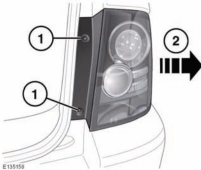
1. With the tailgate open, remove the two screws from the inner edge of the unit.
