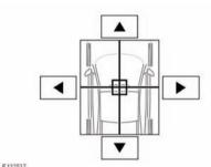
Touch the arrow soft keys to move the sound focal point to the desired area of the vehicle (the focal cross-hairs will appear red when not in the default position).
