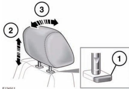
1. Press the locking collar to release the head restraint.
