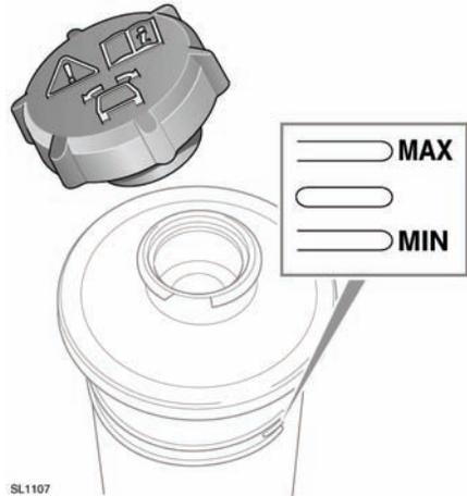
Check the level through the side of the transparent reservoir, without removing the filler cap.
