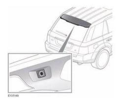
When reverse gear is selected, the screen automatically displays a wide angle, colour image from the rear of your vehicle.
