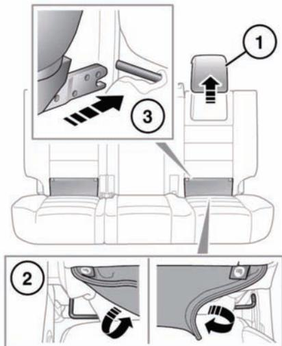
Both of the outer seat positions on the rear seat are equipped to accept ISOFIX restraints.
