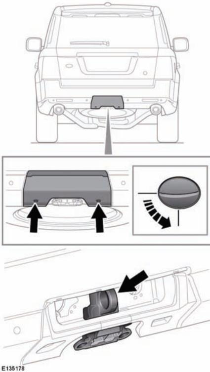
1. Rotate each of the fasteners 90 degrees anticlockwise with a coin (or similar), to release the lower edge.
