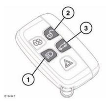
To raise the vehicle press and hold button (1), then press and hold button (2).
