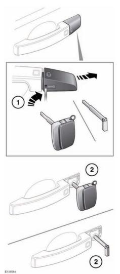
1. Insert the key blade into the slot at the base of the door lock cover and gently lever the key blade upwards.
