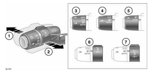
With the headlamps on, push the control away from the steering wheel to select high beam. The instrument pack warning lamp will illuminate.
