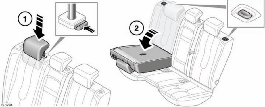
The split fold rear seat of 5 door models can be folded completely, or partially at 60/40 split, to accommodate loads and still retain seating for passengers.
