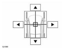
Touch the arrows to move the sound focal point to the desired area of the vehicle. Alternatively, drag the focal point cross hairs to a new position.
