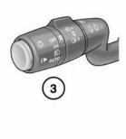
To activate, press the Park Assist button while driving forwards at less than 30km/h (19mph). The indicator lamp in the button illuminates.
