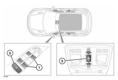
Briefly pull a switch fully up and release, the window will continue to rise until fully closed. Briefly press a switch fully down and release, the window will continue to lower until fully open. Pressing or pulling a switch again will stop the window.
