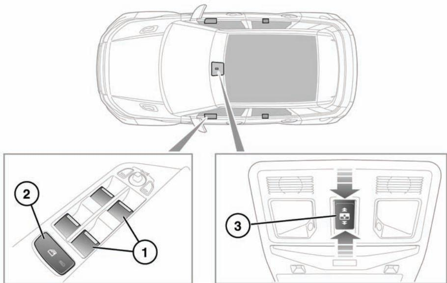
1. Briefly pull a switch fully up and release, the window will continue to rise until fully closed. Briefly press a switch fully down and release, the window will continue to lower until fully open. Pressing or pulling a switch again will stop the window.
