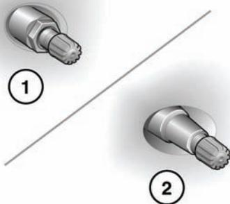
1. TPM system external metal lock nut and valve.
