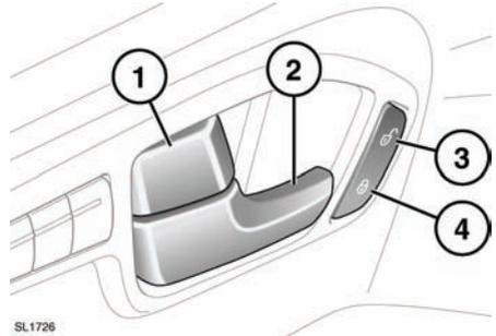
1. Press a locking lever to lock a door. Pull the lever back to unlock. Operating either front door locking levers will lock or unlock all doors.
