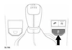
To disable DSC, press and briefly hold the DSC OFF switch. The DSC OFF warning lamp will illuminate continuously. The amber DSC OFF warning lamp in the instrument panel will also illuminate. Deactivating DSC also reduces the level of Electronic Traction Control intervention and may lead to an increase in wheel spin.
