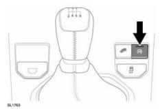
To switch the system off (preventing automatic stop/start) press the **ECO** switch. The LED indicator will extinguish to confirm that the system is off.
