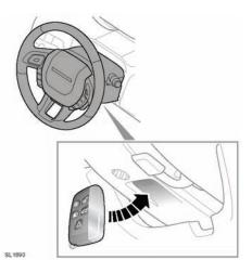
Position the Smart Key against the underside of the steering column cover with the buttons facing downwards.
