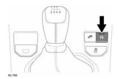
To switch the system off (preventing automatic stop/start) press the **ECO** switch. The LED indicator will extinguish to confirm that the system is off.
