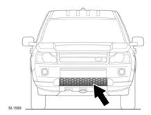
Ensure that the areas around air intakes and the front grille are clean and clear of debris. Pay particular attention to the lower grille and radiator. Failure to do so may cause the engine to overheat, leading to severe engine damage.
