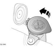
The washer reservoir supplies both front and rear screen washer jets and headlamp washer jets.
