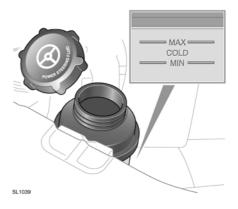
The level of fluid can be seen through the translucent body of the reservoir.
