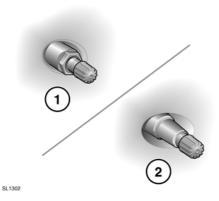
Wheels fitted with a TPM system can be identified by the appearance of the external metal lock nut and valve (1). All Land Rover non-TPM system wheels have a rubber valve fitted (2).
