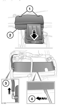
1. Press the clips to release the back of the cover.
