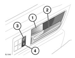
From inside the vehicle, all the doors can be locked by pressing either the driver or passenger lock lever (1).
